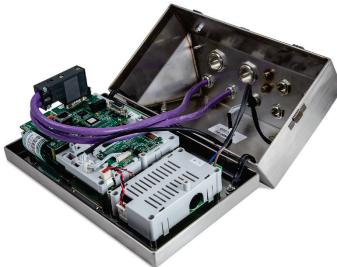
Figure 6-6: Profibus Option Board Installed - Harsh Enclosure
